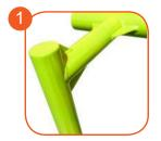
Solid construction made of black steel S235JR, cleaned in the sandblasting process. Protected against corrosion by galvanizing and powder coating with polyester paint QUALICOAT attested.
